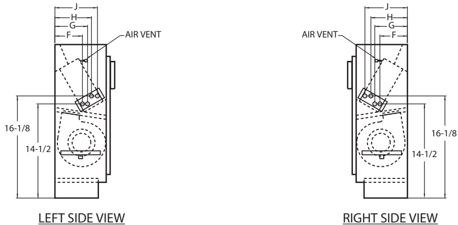
COIL CONNECTION DIMENSIONS (in.)
